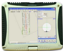
Flight Management System Touchscreen tablet PC in pilot's cabin for realtime position and course control
