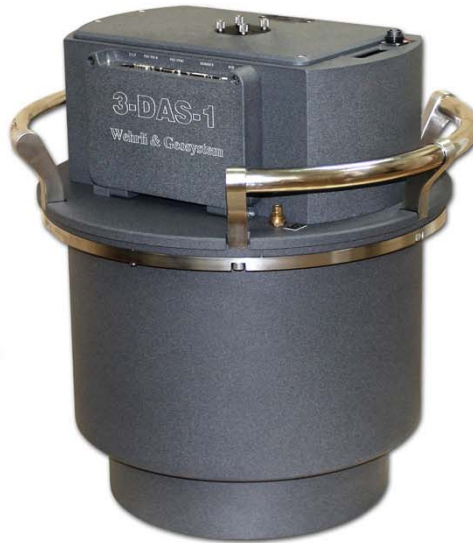
Pushbroom Camera Three RGB-channels 8000 x 9 micron x 42 bit 16°/0°/26°, focal distance 110 mm
